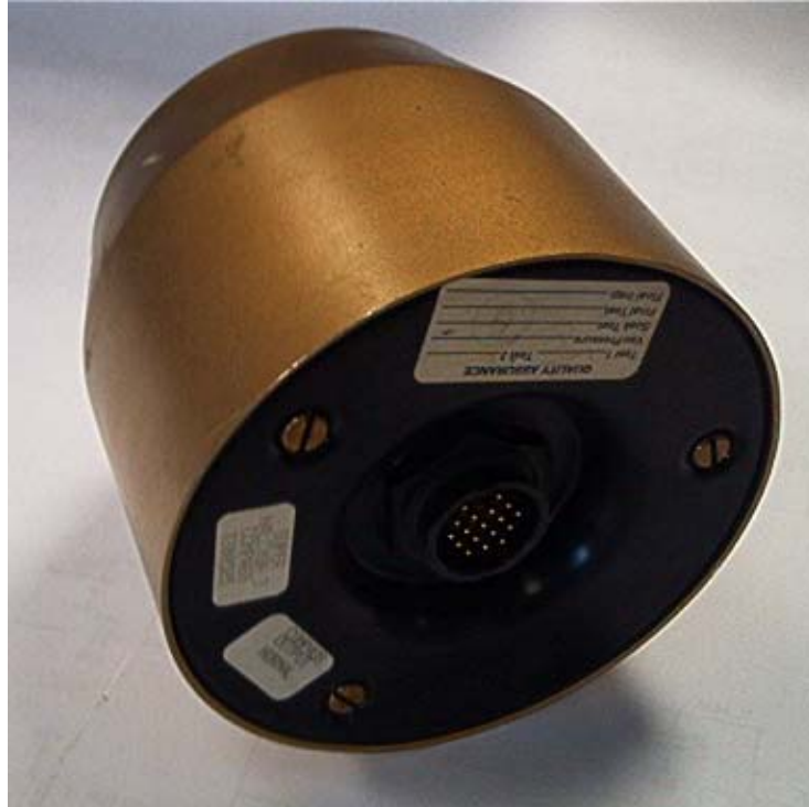
Sensor viewed from the base showing the connector
