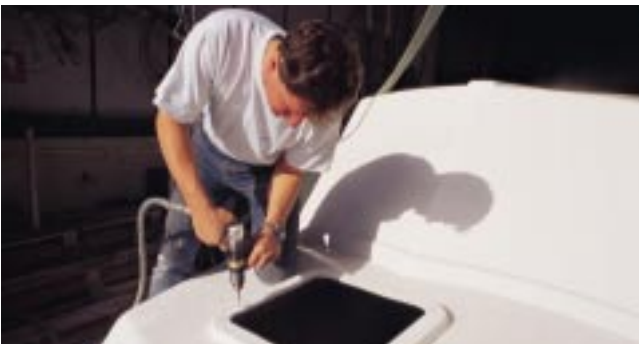
With the hatch removed from the deck drill all fastening holes.
