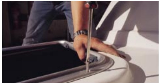
Refit the hatch to the deck. Around the hatch frame a small amount of bedding compound should be forced out of the gap between the frame and deck. Fasten the lower frame to the deck.
