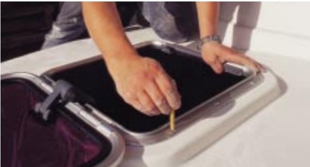
While the hatch is in place mark the lower frame fixing holes.
